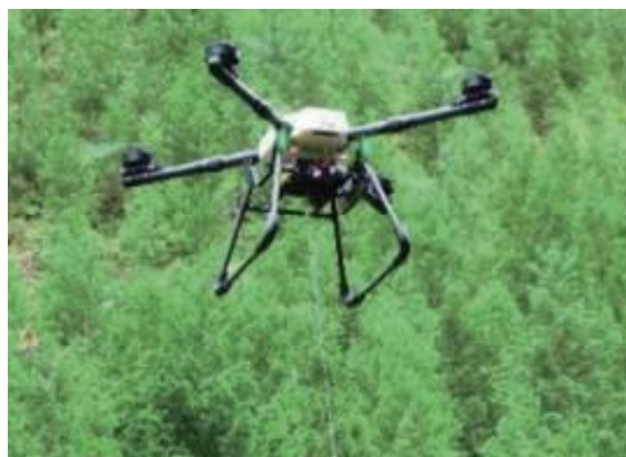
Drone transporting materials for protective fencing
