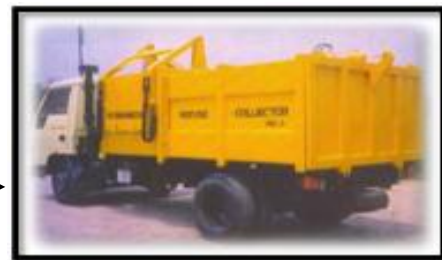
Waste received at 1.1 cum Bins to be transported to SLF by using Refuse Collector
