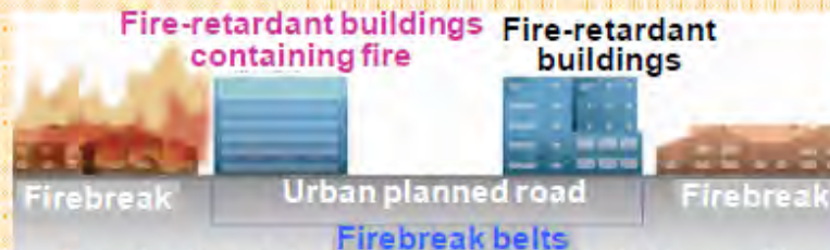
Ensuring the safety of neighboring residential communities Forming firebreak belts (image)
