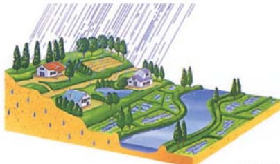
Increased runoff due to urbanization
